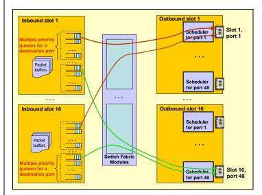
Complementing the large number of virtual output queues is a rich set of scheduling algorithms that can be applied to each Egress port. These mechanisms can either be used individually or in combination to deliver tiered QoS guarantees for several applications on the same port:
