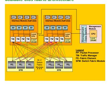
The BigIron RX uses a Clos fabric architecture that provides a high level of scalability, redundancy and performance. As shown in the Figure above, there are multiple switch fabric
